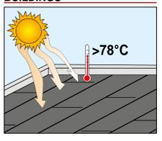
Over 90% of roofs are dark-coloured, and the surface of a roof exposed to solar radiation reaches temperatures of around 80°C, which also has negative effects on the useful life of waterproof coverings.
